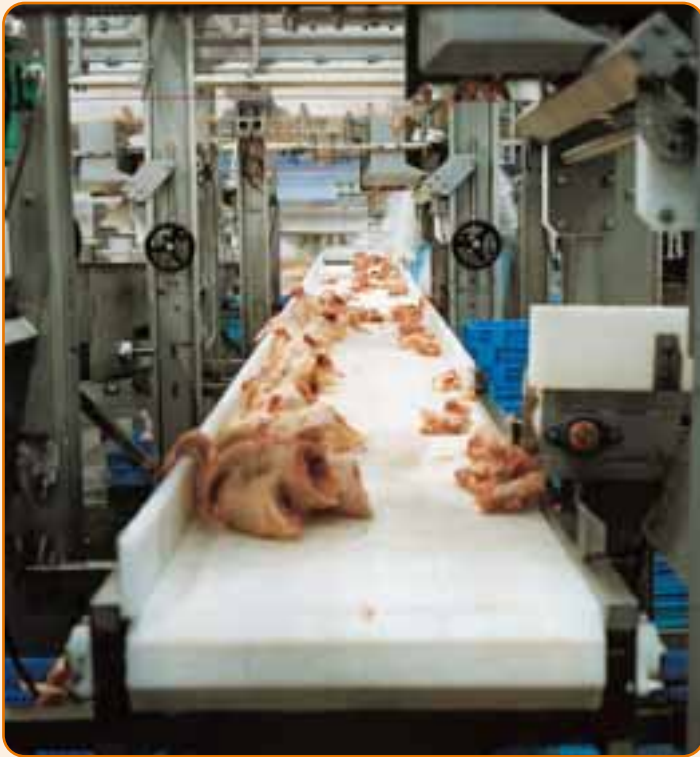
TYPICAL APPLICATION OF A MCC FOOD BELT IN A CHICKEN SLAUGHTER HOUSE
